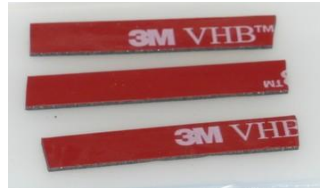
3M VHB Tape to secure wires.
